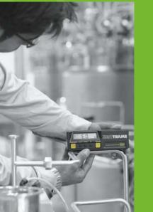
Drainability is an essential feature of any hygienic piping system. Retained fluid in the pipe lines provides a medium where bacteria could grow, adding an unacceptable bioburden to the system. Retained fluid could also promote corrosion, leading to product contamination. The utilization of gravity has been found to be the most effective method of removing all traces of liquid from a process system.
